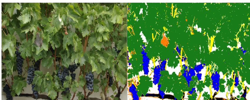
Fig. 1. Original (left) and segmented image (right) of a Tempranillo grapevine canopy in four different classes: clusters, green leaves, yellow-wilted leaves and porosity.
